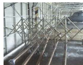
The Jampro JHPC-8 FM Broadcast Antenna ready to be installed
